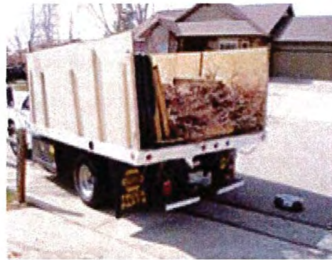
Figure 6: Potentially Unsafely Modified Debris Hauler
